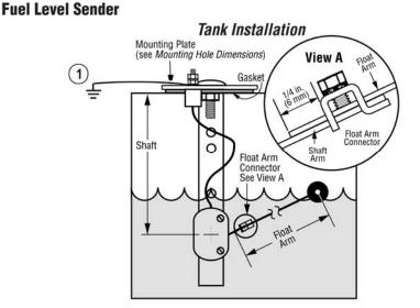
**NOTE:** When installing the fuel sender in a non-metallic tank using a single wire sender, another wire must be added from one of the sender mounting bolts to the battery ground (negative post). See ① in the 'Tank Installation' illustration above.
